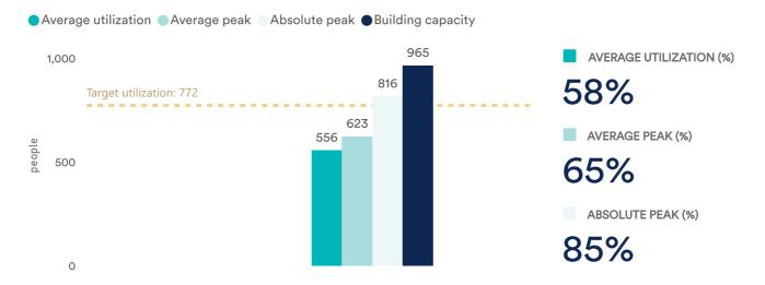
This graph shows the average utilization, the average and absolute peak, alongside the building capacity. These basic insights indicate whether the building is over- or under-utilized.
